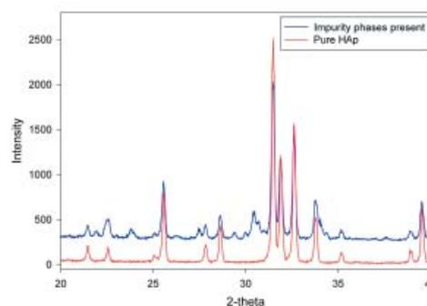
Comparison of x-ray diffraction data from pure HAp and HAp with impurity phases (offset vertically)
