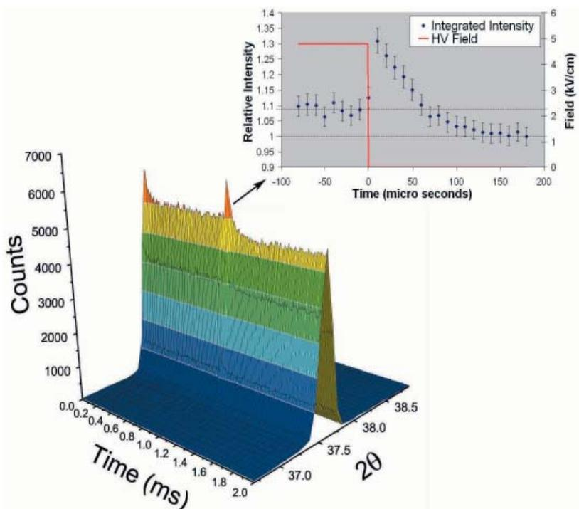
Above: (060) Bragg peak intensity of TGS during the application of a 500Hz square wave, field on from 0-1ms, field off 1-2ms. Data were separated into 200 time frames within the 2ms cycle.
