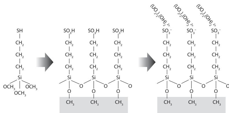
Mercaptopropyltrimethoxysilane (left) is deposited onto a metal oxide substrate and oxidised in order to form a sulphonic acid terminated self-assembled monolayer (middle). Immersed into water, the sulphonic acid group deprotonates and forms a negatively charged surface. Metal cations and their hydrolysed species are electrostatically attracted and immobilised by the surface and can be removed from water (right).
