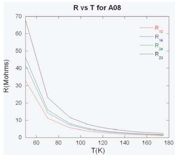
Resistance vs temperature for a tin ion implanted polyetheretherketone sample. The material shows room temperature resistance of  $\sim 1 \text{MW}$ , with a corresponding conductivity of  $\sim 10^{-2} \text{Scm}^{-1}$ . The behaviour (increasing resistance with decreasing temperature) is characteristic of a semiconductor or insulator – not a metal. The 4 curves represent measurements in the 4 Van der Pauw configurations.
