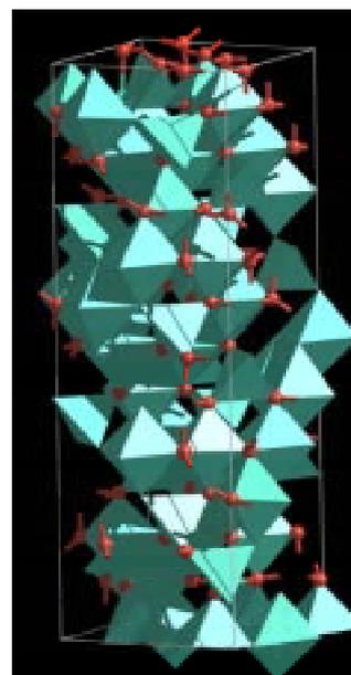
Example  $\gamma$ -alumina structure after optimisation of a possible structural configuration
