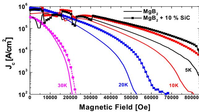
Super-current vs magnetic field for pure and 10 wt % nano-SiC doped MgB<sub>2</sub> made by hot isostatic pressure technique.
