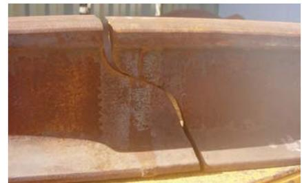
*Close up of a rail which failed in the region of a weld*
