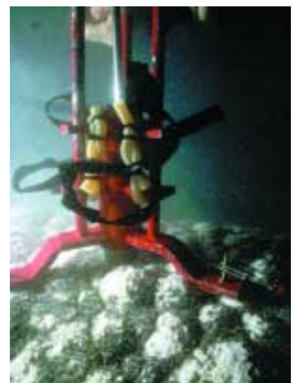
Diver coring submerged calcites.
